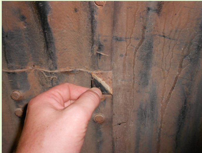
Figure 12. Minor delamination occasionally observed at cut edges. This is expected and has not seemed to be a life-limiting factor.
