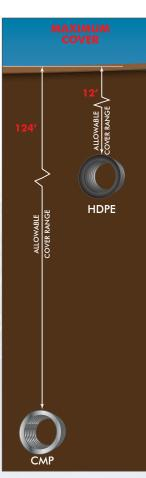
With over 100 years of proven performance, Contech corrugated metal pipe (CMP) solutions offer the best combination of pipe strength and economy for culverts and storm sewers. CMP is available in round and pipe-arch shapes up through 144" diameter and can be manufactured with helical, lock-seam construction or annular corrugations with riveted or spot welded seams. A variety of coupling systems are available to meet the project requirements.
