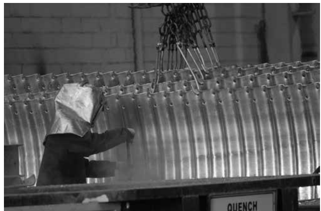
Galvanized MULTI-PLATE removed from the Zinc Tank
