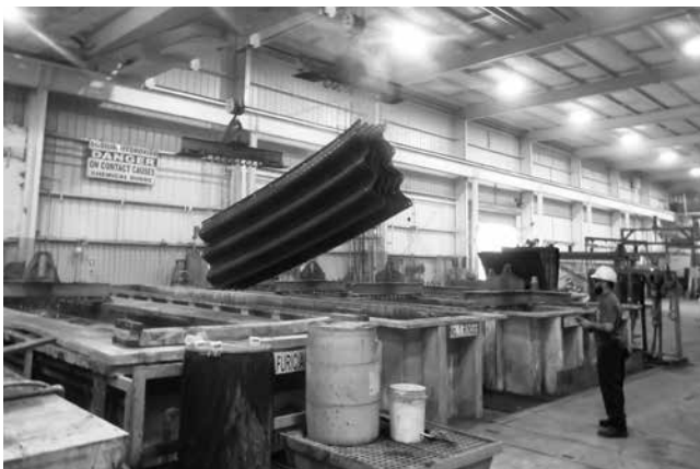
Black Steel MULTI-PLATE before the Zinc Tank
